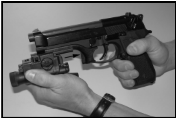
Figure 4: Mounting of the LAM-100 onto the Beretta pistol with adapter.
